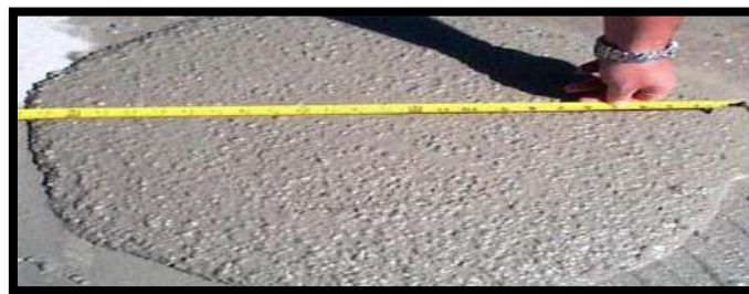
Figure 1: Slump flow test.
